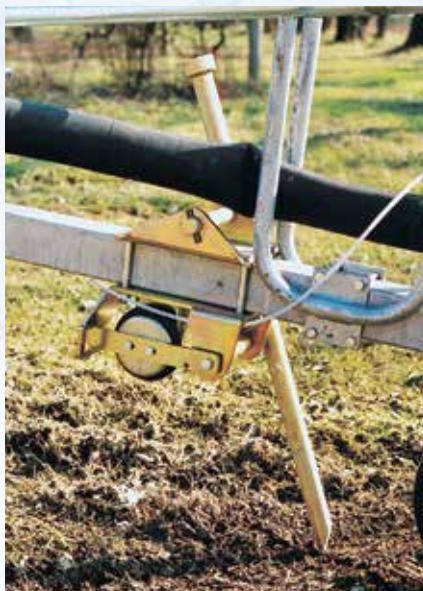
Device for locking trolley to the ground with pickax (for models with rear hose unwinding).
