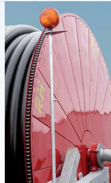
Signal of hose rewind end with xenon arc lamp for RM programmer.
