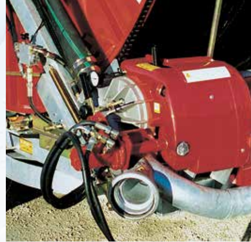
PE hose rewind through hydraulic motor on PTO, speed adjusting valve, limit switch spool valve and quick coupling torque to tractor.
