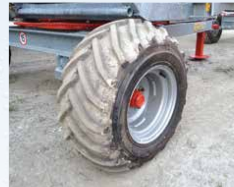
"Big size" type tyre for the 581 Gx Evo model size 26/12.00-12.
