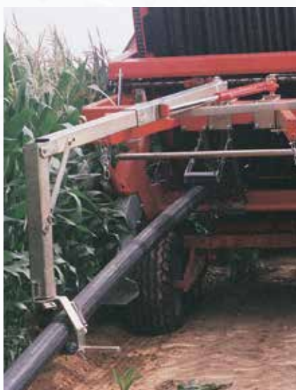
Arm for rear hose unwinding (optional for the 790 Gx, 890 Gx, 990 Gx, 1000 Gx models) and standard on the Magnum Fx.
