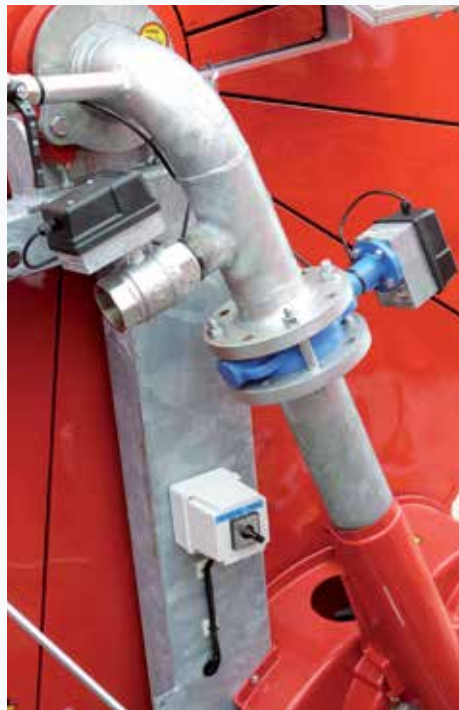
Electromechanical drain valve and electromechanical shut-off valve controlled by programmer (supplied separate or paired and controlled by electric switch).
