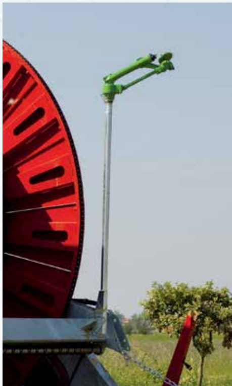
Additional limit switch rain gun controlled by programmer (Skipper or KI model).
