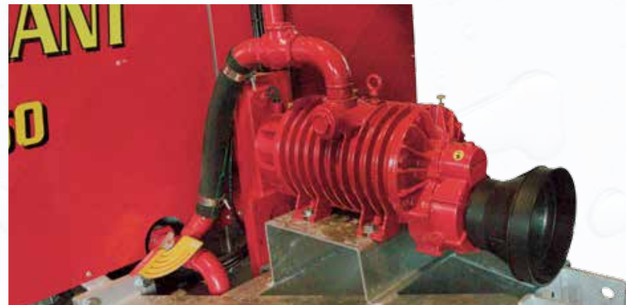
Compressor for emptying the hose JUROP 9000 lt.
