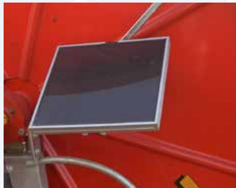
Solar panel for powering electronic equipment.
