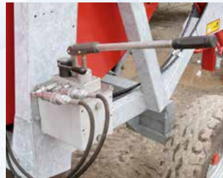
Manual pump for operating rear brackets and lifting trolley (optional for the 570 Gx Evo, 581 Gx Evo, 690 Gx, 790 Gx models).
