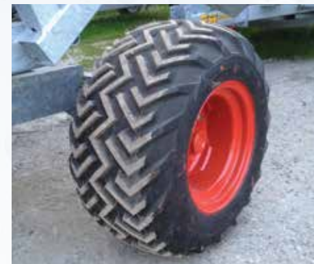
"Big size" type tyre for the 690 Gx Evo and 790 Gx models size 31x15.50-15.
