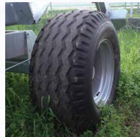
"Big size" type tyre for the 890 Gx, 990 Gx models, standard on the 1000 Gx model (size 15.0/55-17).
