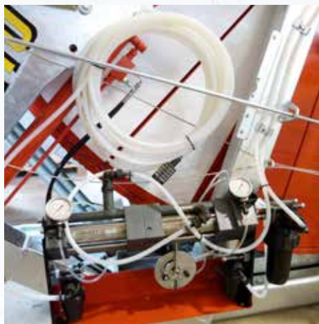
Dosing pump for sewage irrigation with liquid fertilizer.
