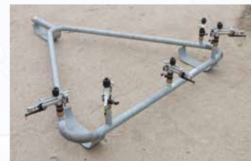
Under-foliage sprinkler device for orchards/vineyards in place of standard trolley.
