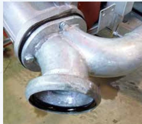
Water inlet on both sides (standard on all the Gx models starting from 581).
