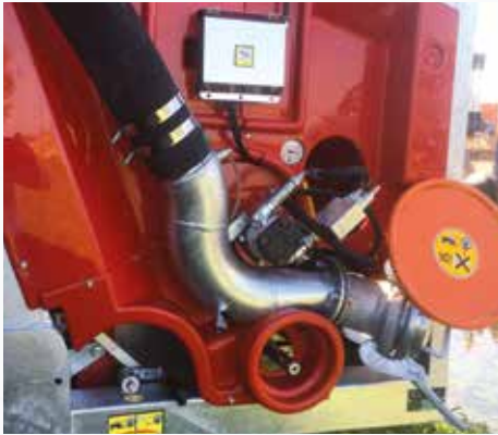
Hose rewind through YANMAR LD70 diesel engine complete with hydrostatic transmission with hydraulic motor on the reduction gear; speed compensating valve, double hydraulic pump for service feed; it can be paired with RM electronic programmers. The optional replaces the turbine rewinding.
