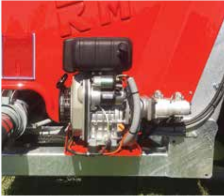
ECU operated by 4-stroke HONDA GX160 engine or by Briggs & Stratton Hp 5.5 for hydraulic services.
