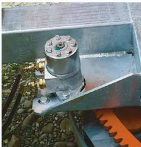
Hydraulic rotation of fifth wheel (standard on all the 990 Gx, 1000 Gx models; optional for all the other models).
