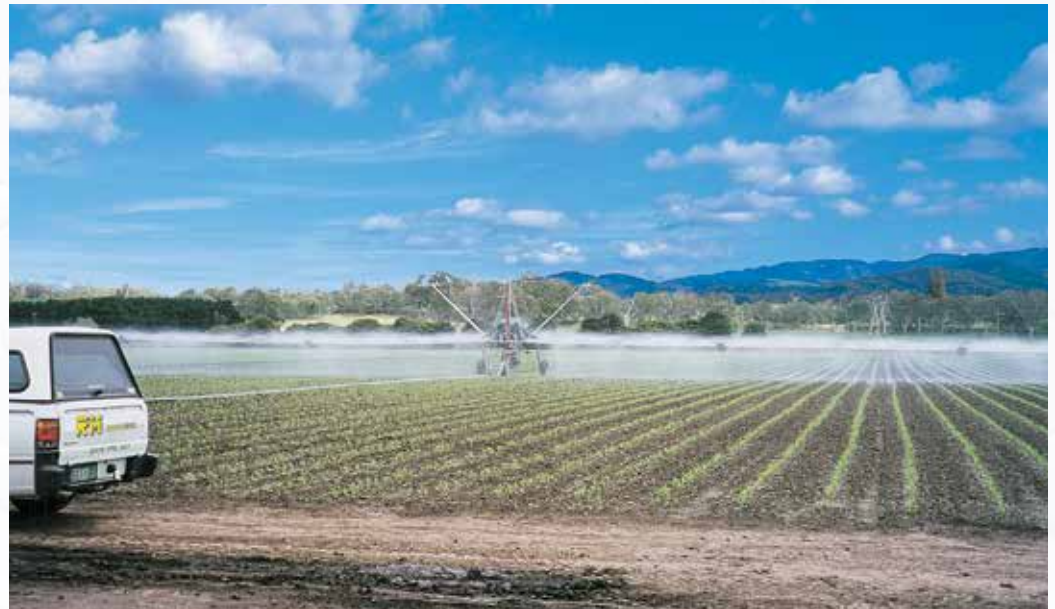
Albatros boom with 72-metre structure (optional for the 990 Gx and 1000 Gx models).
