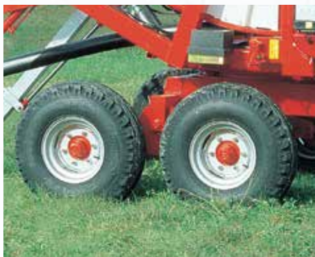
Double axle on asymmetrical rocker arm (optional for the 690 Gx, 790 Gx, 890 Gx models).
