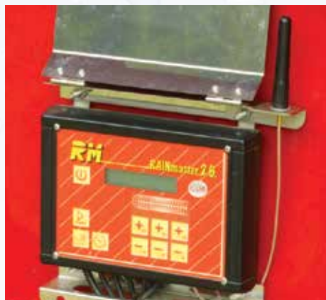
RM programmer; RainMaster 2.6 model (with antenna and in-built optional GSM module).
